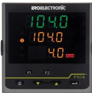
← Measured Temperature (or Process Value 'PV') →
