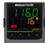
Measured Temperature (or Process Value 'PV') →
