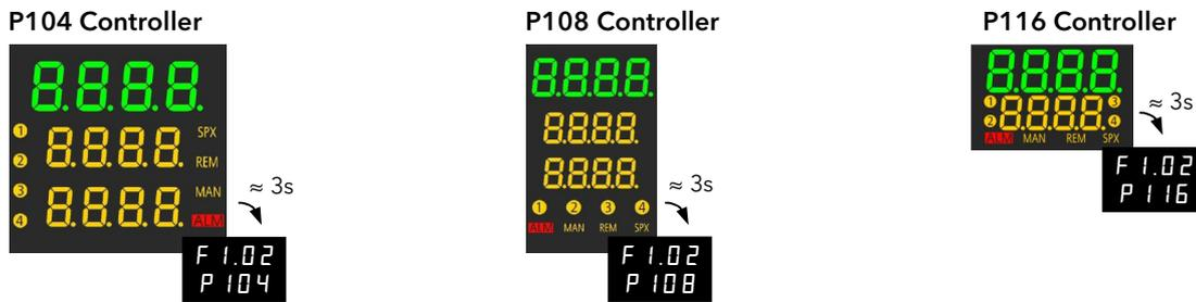
The display that automatically follows depends on the way the controller has been supplied or re-configured and is described in the following sections.
